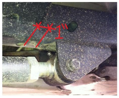
The front frame brackets are spaced back from the existing transmission skid hole by 1" from the rearmost edge of the hole. They should be positioned on the frame so that they are parallel to the centerline of the vehicle. This will cause them to look crooked on the frame. The back edge of the bracket will be flush to the outside of the frame rail while the front edge will stick out from the outside of the frame by about 3/4".
