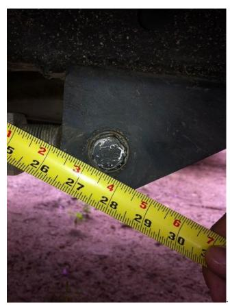
Double-check the position of the front frame bracket by measuring up to the closest edge of the coil/shock bucket. Refer to the position of the end of the tape measure in the picture below. Note that if you had to move the bracket forward because of the length of your flexjoints, this measurement will be different.
