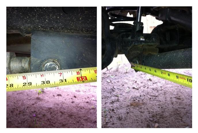
Set the length of the lower arms to 30" from center of the front bushing to the center of the flex-joint and install the lower arms. The measurement shown is taken from the front of the forward mounting bolt. See the right photo.
